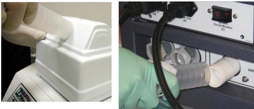
**NOTE** For optimal evacuation of aerosols, ensure that the tubing is securely connected at both ends.
