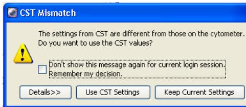
By selecting Use CST Settings, the laser delay, area scaling, and other cytometer settings will be updated to the latest optimized settings from the performance check.
