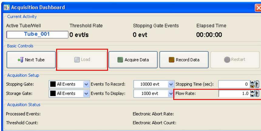
Note that the relatively longer sample tubing on the BD FACSAria II cytometer results in a different flow rate between cells and beads. Thus, absolute counting using BD Trucount™ beads can yield erroneous results.
