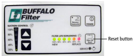
The green and amber LED lights will turn off, and then on. Hold down the button until the 100% indicator light is lit. This resets the 180-hour filter life clock.
